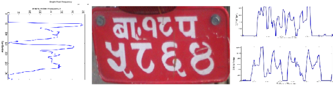
Fig. 4: Row profile in the left, localized image in the center and column profile of two blocks of characters in the right.
